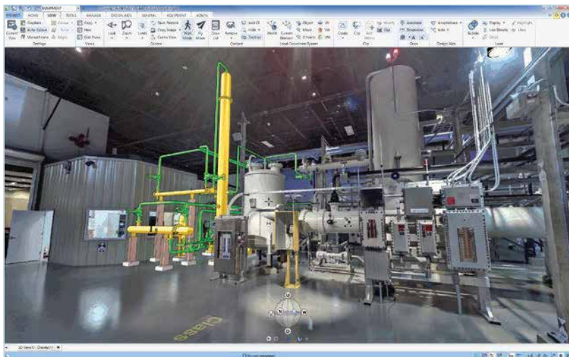
Laser scan data integrated into the 3D view
